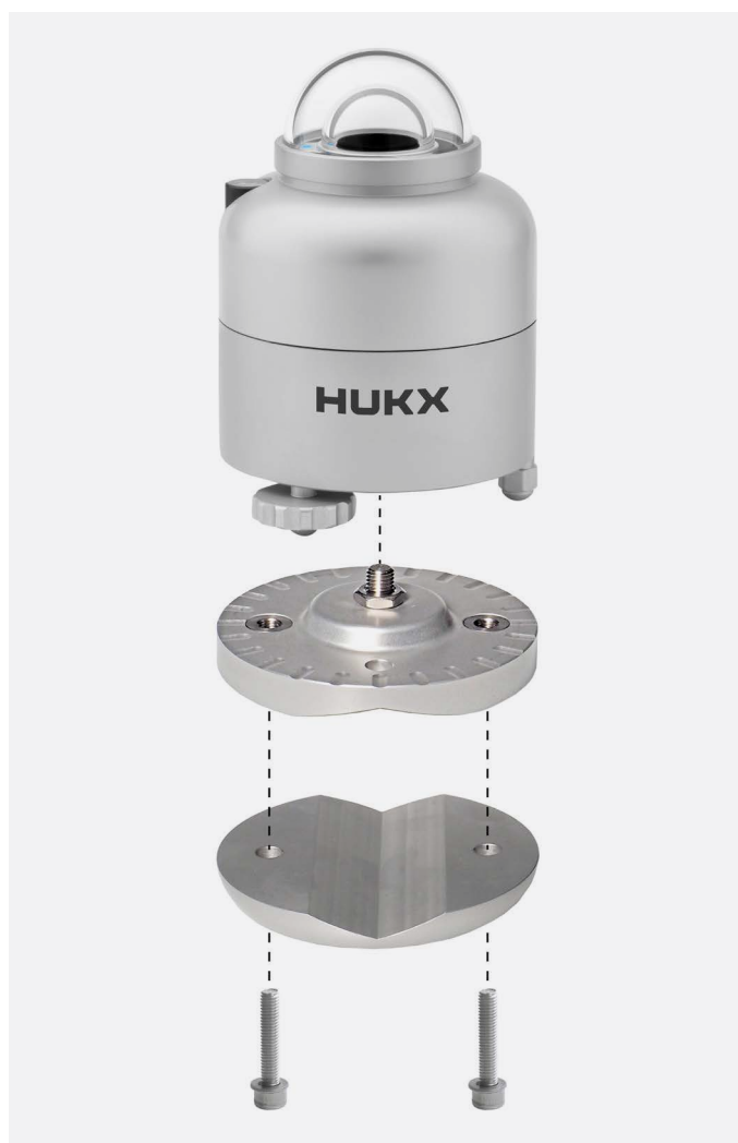
Figure 5 Optional LM01 spring-loaded leveling mount (one part) and TLM01 tube leveling mount (2 parts) for SR300-D1, SR200-D1, and SR100-D1. Spring-loaded leveling is a major time-saver during installation.
